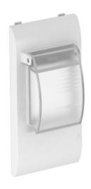
Construction set, protection unit installation consisting of cover with mounting support and transparent cover hood. Allows the installation of protective equipment (two units) such as miniature circuit-breakers or FI protection switches in the Modalnet housing.
