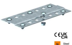
Wide joint plate for use in all cable trays and wide span cable trays. Including appropriate fastening material. For function maintenance at a width of 100 mm, the quantity of supplied M6 truss-head bolts should be increased to four, whilst for widths 200 and 300 mm, it should be increased to six.
