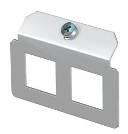
Support plate to accept two data connection sockets, type Panduit in combination with Panduit adapter CMNZABL-X or CMNZAWH-X. Dimensions of a mounting opening in mm: 19.8 x 21.2.
