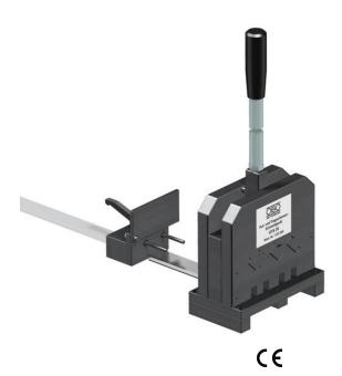
With the HTS 35 hat and support rail cutting device, you can cut the four most common hat and support rail profiles (types 2069..., 46277... and 2064...) to fit and without burring in accordance with DIN 50022 and DIN 50035.
