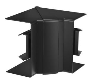
Internal corner cover made of halogen-free PC/ABS for changing the direction of Rapid 80 device installation trunking of the GK, GKH, GS and GA systems. The fittings can be variably adjusted between 85° and 95° and can be used in symmetrical and asymmetrical trunking.
