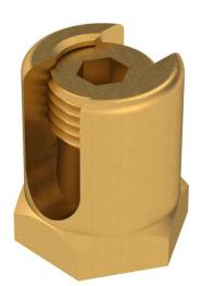
Earthing terminal for fastening the equipotential bonding conductor to the cable support system. M14 threaded pin, Allen drive with 6 mm across flats.
