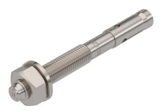
Bolt tie BZ3 for the anchoring of medium-duty to heavy-duty loads, both in cracked and non-cracked concrete. Suitable for heavy loads with small edge and axial distances. For knocking in.
