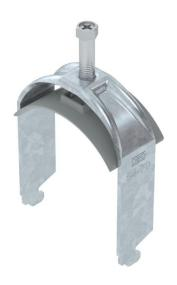
Clamp clip with N-foot, plastic pressure sleeve made of polypropylene. For vertical and horizontal mounting of 1 single cable on a C-profile rail. For slot width 11–12 mm With 1-start screw thread on pressure sleeve, universal hexagonal screw head WAF10, with slot and cross recess. Suitable for assembly indoors and outdoors. We recommend the use of a counter-sleeve.
