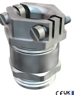
Cable gland with centrically acting transverse clip strain relief in the pressure screw, bend protection of movable cables through strongly rounded pressure screw.
